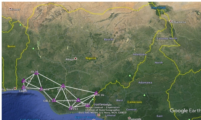
Figure 3. Map of the Campaign GNSS Triangulation Network in Southern States of Nigeri, [Authors]
