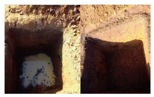
Figure 2b. Pictures of Test Pits (TP1 and TP5 respectively)
