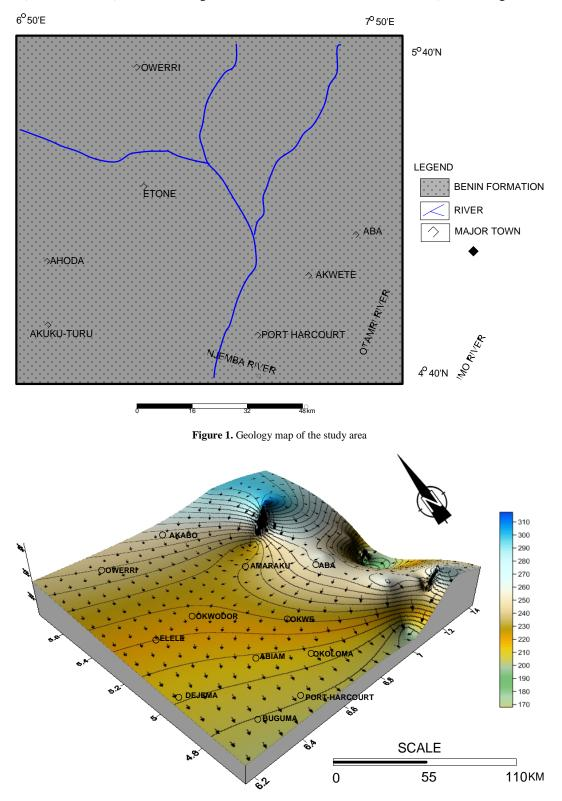
Figure 2. Digital terrain model of the study area overlapped with contour and flow lines
