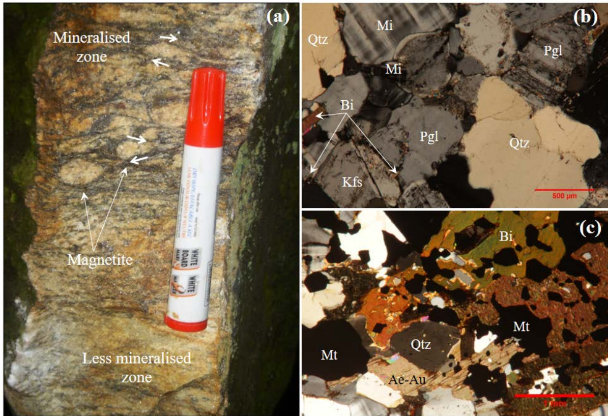
Figure 3. (a) Representative sample and photomicrographs of the magnetite-biotite gneiss showing texture, deformation and distribution of minerals in the rocks. White arrows presents shear orientation. Notice the augen texture. (b)-(c) Transmitted light photomicrographs showing the mineralogical composition of the magnetite-biotite gneiss. Qtz; quartz, Mi: microcline, Bi: biotite, Pgl: plagioclase, Kfs: potassic feldspar, Mt: magnetite, Ae-Au: aegerine - augite
