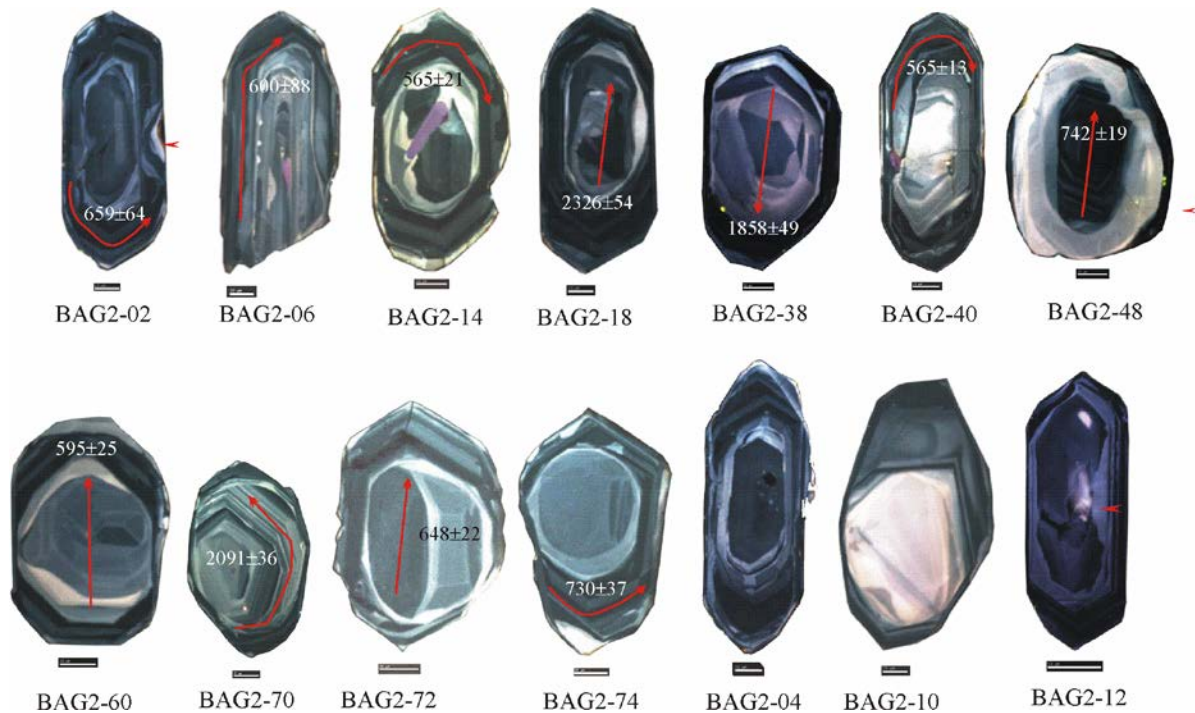
Figure 6. Cathodoluminescence images of selected zircons of the BMG (sample BAG2). The arrows show the approximate location of the laser ablation trenches
