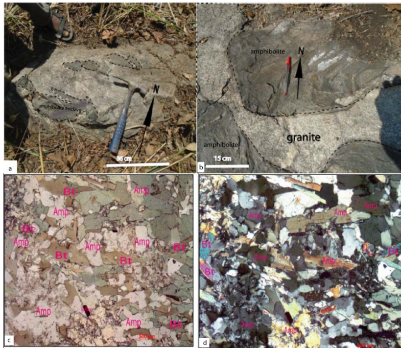
Figure 3. a- Amphibolite enclave in an orthogneiss slab; b- Amphibolite septa in orthogneiss affected by granite; c- Granonematoblastic texture of amphibolites in LPNA, d- Granonematoblastic texture of amphibolites in LPA
